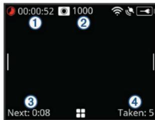
The camera takes a series of photos at the selected interval. The screen displays the elapsed time **1**, the remaining number of photos the camera can take **2**, the time in seconds until the next photo is taken **3**, and the number of photos the camera has taken in
